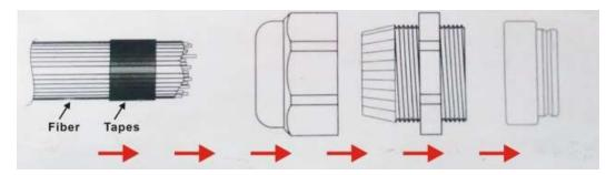
3. Cut the fibre bundle to a flat surface with a heat-knife or blade.
