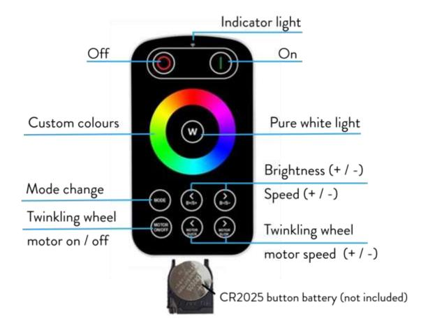
The light engine can be controlled by the remote controller and the Bluetooth App at the same time.
